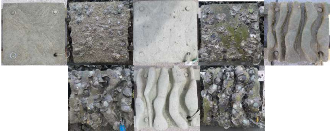
Figure 2. Month 1 and 12 comparison of (Upper row, clockwise) seawall, flat, 2.5 cm, 5 cm plates.
